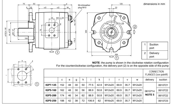
NOTE 5: For applications with delivery pressure > 200 bar, a special connection flange cod. 0610725 is required.
