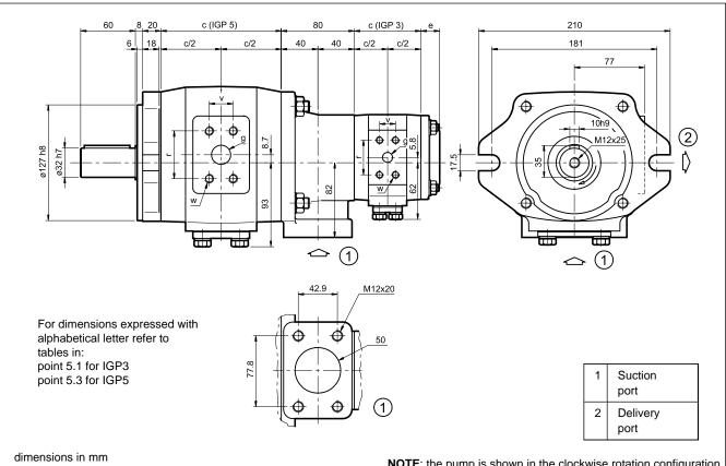
**NOTE**: the pump is shown in the clockwise rotation configuration For the counterclockwise configuration, the delivery port (2) is on the opposite side of the pump
