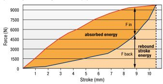
With the aid of the characteristic curves above you can estimate the proportion of the total energy that will be absorbed. Example: With impact energy of 50 Nm the Energy-Stroke diagram shows that a stroke of about 8.8 mm is needed. On the Force-Stroke diagram you can estimate the proportion of absorbed energy to rebound energy at this stroke length. **Dynamic (v > 0.5 m/s) and static (v \leq 0.5 m/s) characteristics of all types are available on request.**
