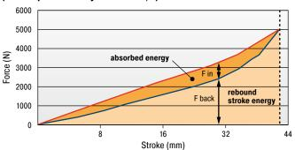
With the aid of the characteristic curves above you can estimate the proportion of the total energy that will be absorbed. Example: With impact energy of 50 Nm the Energy-Stroke diagram shows that a stroke of about 31 mm is needed. On the Force-Stroke diagram you can estimate the proportion of absorbed energy to rebound energy at this stroke length. **Dynamic (v > 0.5 \text{ m/s}) and static (v \le 0.5 \text{ m/s}) characteristics of all types are available on request.**
