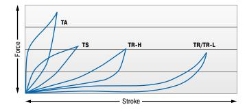
Characteristics of dynamic energy absorption for impact velocity over 0.5 m/s.
