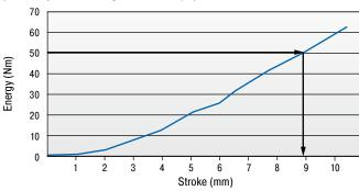
Type TA37-16 Force-Stroke Characteristic (dynamic) (with impact velocity over 0.5 m/s)
