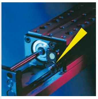
Miniature Shock Absorber in compact pneumatic module
