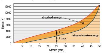
With the aid of the characteristic curves above you can estimate the proportion of the total energy that will be absorbed. Example: With impact energy of 50 Nm the Energy-Stroke diagram shows that a stroke of about 25 mm is needed. On the Force-Stroke diagram you can estimate the proportion of absorbed energy to rebound energy at this stroke length. **Dynamic (v > 0.5 \text{ m/s}) and static (v \le 0.5 \text{ m/s}) characteristics of all types are available on request.**
