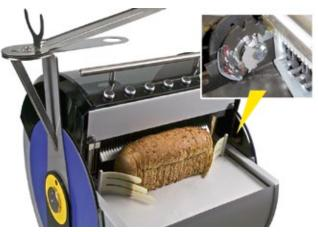
Protective flaps secured with rotary dampers: the simple operation of bread slicing machines can then be easily managed by hand Daub Bakery Machinery BV, 5050 AB Goirle, Netherlands
