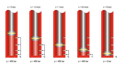
\* The load velocity reduces continously as you travel through the stroke due to the reduction in the number of metering orifices (\*) in action. The internal pressure remains essentially constant and thus the force vs. stroke curve remains linear.
