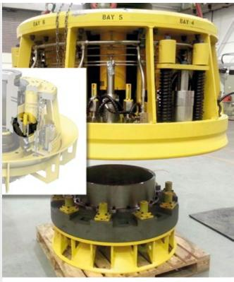
MAGNUMS allow for emergency quick disconnection of the pipelines from the oil rigs
