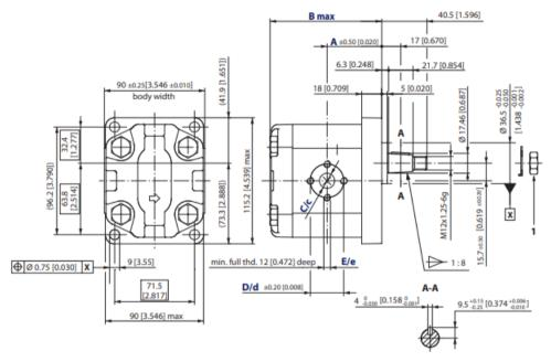
1. Nut and washer supplied with pump; recommended tightening torque 45-55 N·m.
