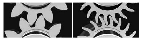
The comparison between the flow characteristic of Danfoss SKP2 (11-teeth) and shhark® (17-teeth) is illustrated in the plot below: the reduction of peak-to-peak flow pulsation is 78%. In addition, the average flow per unit width of shhark® is approximately 2.7% higher than SKP2; this means that for the exact same pump dimensions, shhark® delivers more flow.
