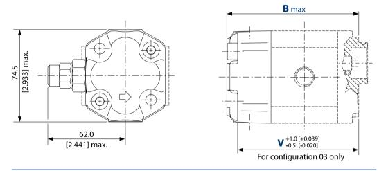
For configuration 06 (SAE A-A) dimension B and V have to be increased 4.5 mm [0.177 in].
