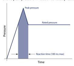
**Rated pressure** is the average, regularly occurring, operating pressure that should yield satisfactory product life. The maximum machine load demand determines rated pressure. For all systems, the load should move below this pressure.
