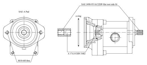
Dimensions for SNP2NN / 06SL flange/shaft option with auxiliary mounting pad kit installed
