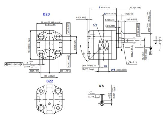
1. Nut and washer supplied with pump; recommended tightening torque 45-55 N·m.
