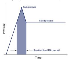
**Rated pressure** is the average, regularly occurring, operating pressure that should yield satisfactory product life. The maximum machine load demand determines rated pressure. For all systems, the load should move below this pressure.
