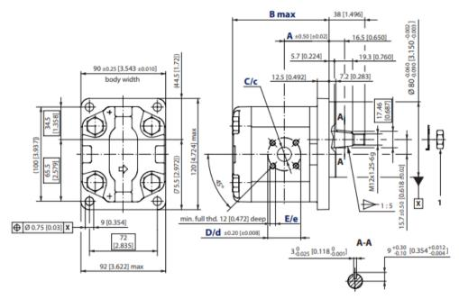
1. Nut and washer supplied with pump; recommended tightening torque 45-55 N·m.
