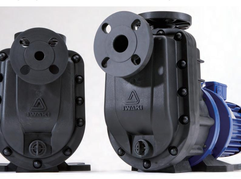
The SMX-F is a horizontal self-priming magnetic drive pump made from fluororesin. Our original self-radiation structure enhances resistance to dry running, cavitation, and closed-discharge operation. In addition, the use of standard motors extends the range of application.
