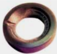
eroded ball seat
