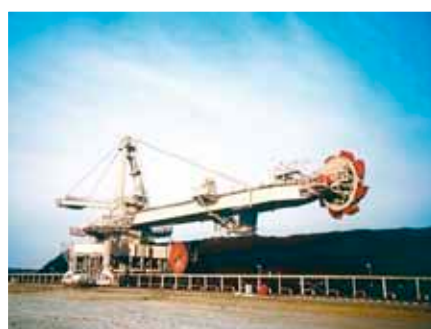
Stacker and reclaimer
