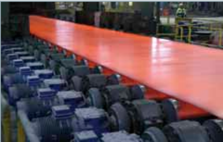
5 Rougher exit roller table
