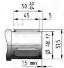
**Gear reducer hollow shaft with keyway**
