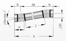
Α Overall length ZA mm AB AB = (A - 2xN)mm Tube length Ζ mm Z = (A - 2xH)
