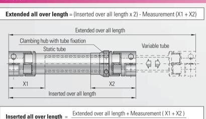
The extended over all length and the inserted over all length are related. Depending on the requirements, the coupling length can be calculated using the two formulas shown here to receive the extended or the inserted over all length.
