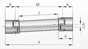
Overall length m ΑB Length AB = (A - 2xN)m Tube length Ζ m Z = (A - 2xH)Н Length of the coupling mm Ν Distance between center lines mm Max. torque NmAngle of twist degree Torsional stiffness of both elastomer inserts Nm/rad  $C_{\tau}^{ZWR}$ Torsional stiffness of tube Nm/rad per meter  $C_{\text{Tdyn}}{}^{\text{EZ}}$ Torsional stiffness of entire coupling Nm/rad
