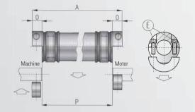
Mounting: Loosen Screw E and slide the metal bellows coupling segments onto each shaft end. Now insert the intermediate tube and assemble onto both metal bellows coupling segments using the assembly screws J. Tighten the assembly screws J to the correct torque indicated in the specification table. Center the entire line shaft coupling onto the shaft ends and tighten screw E by using a torque wrench to ensure the correct torque as indicated in the specification table.
