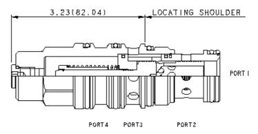
The direct-acting reducer/reliever main section is meant to act as an interface between a low flow pressure source at port 4 and a circuit with higher flow requirements. The valve will reduce a high primary pressure at the inlet (port 2) to a reduced pressure at port 1, with a full-flow relief function from port 1 to tank (port 3).
