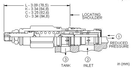
Direct-acting, pressure reducing/relieving valves reduce a high primary pressure at the inlet (port 2) to a constant reduced pressure at port 1, with a full-flow relief function from port 1 to tank (port 3). These valves incorporate a damped construction for stable operation allowing the use of high reduced pressure.
