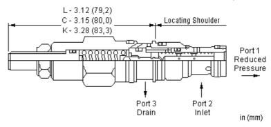
Direct-acting, pressure reducing valves reduce a high primary pressure at the inlet (port 2) to a constant reduced pressure at port 1. These valves incorporate a damped construction for stable operation allowing the use of high reduced pressure. This valve is open in the transition from reducing to relieving. It provides good pressure control and dynamic response.
