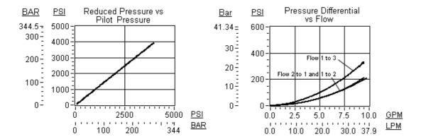
SERIES 2 / CAPACITY: 80 L/min. / CAVITY: T-22A
