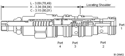
Ventable, pilot-operated pressure reducing/relieving valves reduce a high primary pressure at the inlet to a constant reduced pressure at port 1, with a full-flow relief function from port 1 to tank (port 3). The vent port (port 4) can be used as a means for remote control by pilot or 2-way valves.
