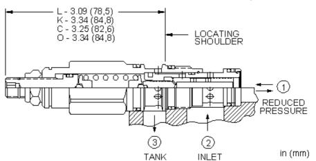
Direct-acting, pressure reducing valves reduce a high primary pressure at the inlet (port 2) to a constant reduced pressure at port 1. These valves incorporate a damped construction for stable operation allowing the use of high reduced pressure. This valve is open in the transition from reducing to relieving. It provides good pressure control and dynamic response.
