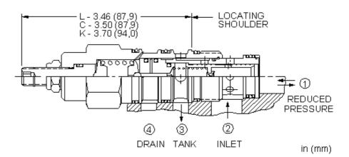
Externally drained, pilot-operated pressure reducing/relieving valves reduce a high primary pressure at the inlet (port 2) to a constant reduced pressure at port 1, with a full-flow relief function from port 1 to tank (port 3). Draining the pilot section at port 4 makes these valves insensitive to pressure at tank (port 3) and provides a means for remote control by pilot or 2-way valves.
