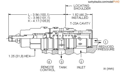
Ventable, pilot-operated pressure reducing/relieving valves reduce a high primary pressure at the inlet to a constant reduced pressure at port 1, with a full-flow relief function from port 1 to tank (port 3). The vent port (port 4) can be used as a means for remote control by pilot or 2-way valves.
