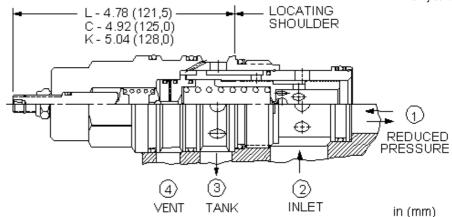
Ventable, pilot-operated pressure reducing/relieving valves reduce a high primary pressure at the inlet to a constant reduced pressure at port 1, with a full-flow relief function from port 1 to tank (port 3). The vent port (port 4) can be used as a means for remote control by pilot or 2-way valves.
