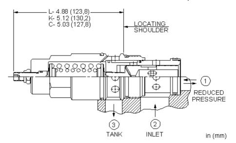
Direct-acting, pressure reducing/relieving valves reduce a high primary pressure at the inlet (port 2) to a constant reduced pressure at port 1, with a full-flow relief function from port 1 to tank (port 3). These valves incorporate a damped construction for stable operation allowing the use of high reduced pressure.
