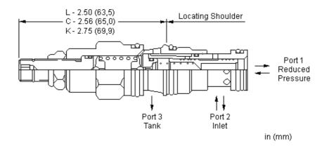
Pilot-operated, pressure reducing/relieving valves reduce a high primary pressure at the inlet (port 2) to a constant reduced pressure at port 1, with a full-flow relief function from port 1 to tank (port 3).
