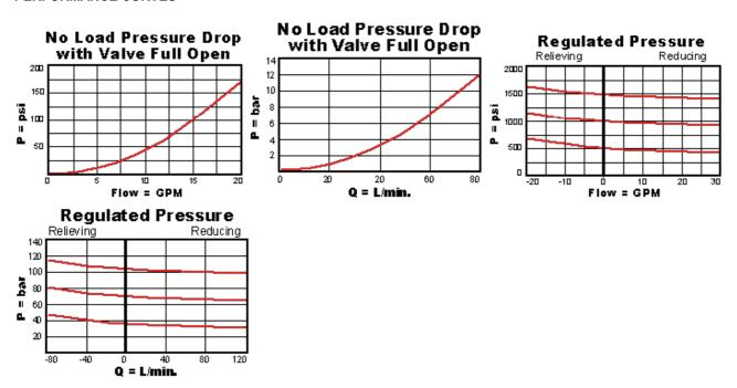
SERIES 3 / CAPACITY: 160 L/min. / CAVITY: T-23A
