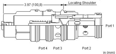
The direct-acting reducer/reliever main section is meant to act as an interface between a low flow pressure source at port 4 and a circuit with higher flow requirements. The valve will reduce a high primary pressure at the inlet (port 2) to a reduced pressure at port 1, with a full-flow relief function from port 1 to tank (port 3).
