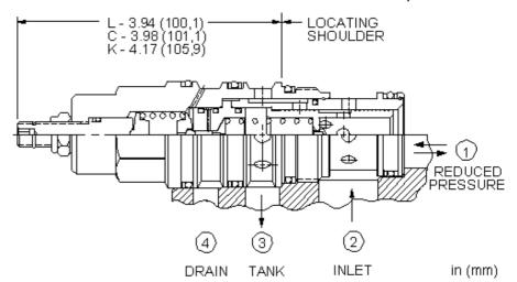
Externally drained, pilot-operated pressure reducing/relieving valves reduce a high primary pressure at the inlet (port 2) to a constant reduced pressure at port 1, with a full-flow relief function from port 1 to tank (port 3). Draining the pilot section at port 4 makes these valves insensitive to pressure at tank (port 3) and provides a means for remote control by pilot or 2-way valves.
