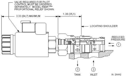
This valve is a 3-way, normally open modulating element that incorporates an integral pilot control cavity. The pilot control cavity will accept any T-8A pressure control cartridge. The valve reduces a high primary pressure at the inlet (port 2) to a constant reduced pressure at port 1, with a full flow relief function from port 1 to tank (port 3). The pilot cartridge's setting determines the difference in pressure between reduced pressure (port 1) and the tank (port 3).
