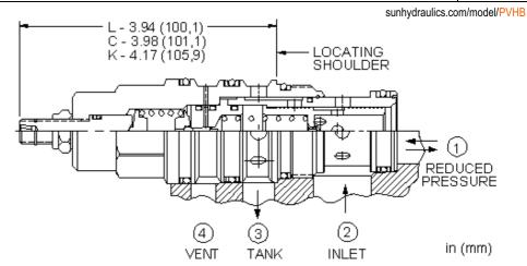
Ventable, pilot-operated pressure reducing/relieving valves reduce a high primary pressure at the inlet to a constant reduced pressure at port 1, with a full-flow relief function from port 1 to tank (port 3). The vent port (port 4) can be used as a means for remote control by pilot or 2-way valves.
