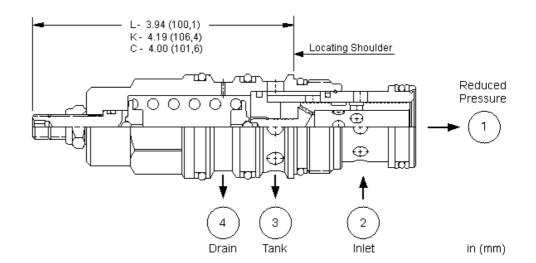
Direct-acting, pressure reducing/relieving valves reduce a high primary pressure at the inlet (port 2) to a constant reduced pressure at port 1, with a full-flow relief function from port 1 to tank (port 3). Draining port 4 makes the valve insensitive to pressure at port 3. These valves incorporate a damped construction for stable operation allowing the use of high reduced pressure.
