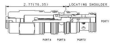
The direct-acting reducer/reliever main section is meant to act as an interface between a low flow pressure source at port 4 and a circuit with higher flow requirements. The valve will reduce a high primary pressure at the inlet (port 2) to a reduced pressure at port 1, with a full-flow relief function from port 1 to tank (port 3).
