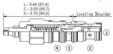
Direct-acting, pressure reducing/relieving valves reduce a high primary pressure at the inlet (port 2) to a constant reduced pressure at port 1, with a full-flow relief function from port 1 to tank (port 3). Draining port 4 makes the valve insensitive to pressure at port 3. These valves incorporate a damped construction for stable operation allowing the use of high reduced pressure.
