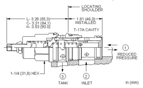
Pilot-operated, pressure reducing/relieving valves reduce a high primary pressure at the inlet (port 2) to a constant reduced pressure at port 1, with a full-flow relief function from port 1 to tank (port 3).
