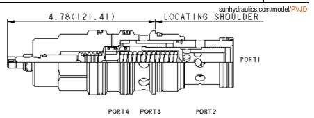
Ventable, pilot-operated pressure reducing/relieving valves reduce a high primary pressure at the inlet to a constant reduced pressure at port 1, with a full-flow relief function from port 1 to tank (port 3). The vent port (port 4) can be used as a means for remote control by pilot or 2-way valves.
