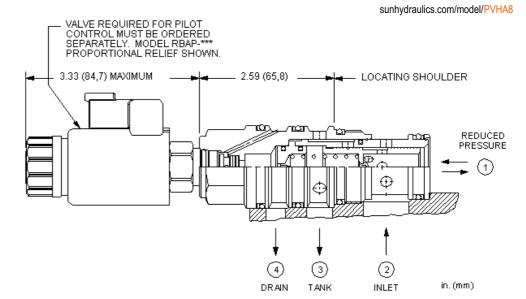
This valve is a 3-way, normally open modulating element, externally drained, that incorporates an integral pilot control cavity. The pilot control cavity will accept any T-8A pressure control cartridge. The valve reduces a high primary pressure at the inlet (port 2) to a constant reduced pressure at port 1, with a full flow relief function from port 1 to tank (port 3). The pilot cartridge's setting determines the difference in pressure between reduced pressure (port 1) and the drain (port 4).
