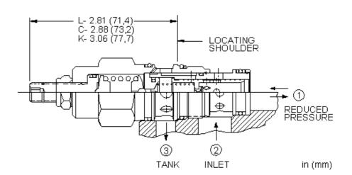
Pilot-operated, pressure reducing/relieving valves reduce a high primary pressure at the inlet (port 2) to a constant reduced pressure at port 1, with a full-flow relief function from port 1 to tank (port 3).
