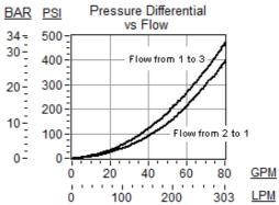
SERIES 1 / CAPACITY: 40 L/min. / CAVITY: T-21A
