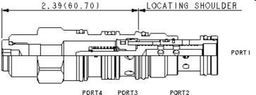
The direct-acting reducer/reliever main section is meant to act as an interface between a low flow pressure source at port 4 and a circuit with higher flow requirements. The valve will reduce a high primary pressure at the inlet (port 2) to a reduced pressure at port 1, with a full-flow relief function from port 1 to tank (port 3).
