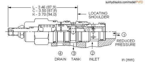
Ventable, pilot-operated pressure reducing/relieving valves reduce a high primary pressure at the inlet to a constant reduced pressure at port 1, with a full-flow relief function from port 1 to tank (port 3). The vent port (port 4) can be used as a means for remote control by pilot or 2-way valves.
