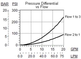
SERIES 3 / CAPACITY: 160 L/min. / CAVITY: T-23A
