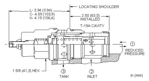
Pilot-operated, pressure reducing/relieving valves reduce a high primary pressure at the inlet (port 2) to a constant reduced pressure at port 1, with a full-flow relief function from port 1 to tank (port 3).
