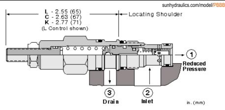
Pilot-operated, pressure reducing valves reduce a high primary pressure at the inlet (port 2) to a constant reduced pressure at port 1, allowing circuits with multiple pressure requirements to be operated using a single pump.
