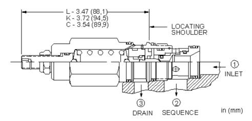
Direct-acting sequence valves will supply a secondary circuit with flow once the pressure at the inlet (port 1) has exceeded the valve setting. The pressure setting of a sequence valve controls the pressure at port 1 relative to the pressure at the drain (port 3).
