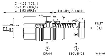
Pilot-operated, balanced poppet sequence valves will supply a secondary circuit with flow once the pressure at the inlet (port 1) has exceeded the valve setting. The pressure setting of a sequence valve controls the pressure at port 1 relative to the pressure at the drain (port 3). These valves are insensitive to back pressure at port 2 (sequence), up to the valve setting. They may be used to regulate pressure in place of 2-port relief valves if there is pressure in the return line.
