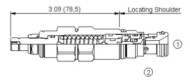
Atmospherically referenced, direct-acting sequence valves will supply a secondary circuit with flow once the pressure at the inlet (port 1) has exceeded the valve setting. The pressure setting of this sequence valve controls the pressure at port 1 relative to the atmospheric vent.
