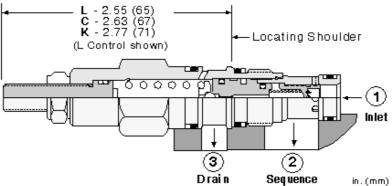
Pilot-operated, balanced piston sequence valves will supply a secondary circuit with flow once the pressure at the inlet (port 1) has exceeded the valve setting. The pressure setting of a sequence valve controls the pressure at port 1 relative to the pressure at the drain (port 3). These valves are insensitive to back pressure at port 2 (sequence), up to the valve setting. They may be used to regulate pressure in place of 2-port relief valves if there is pressure in the return line.
