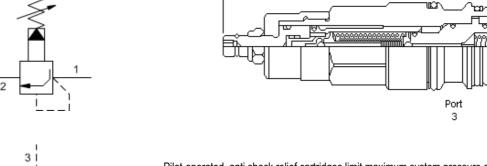
Pilot-operated, anti shock relief cartridges limit maximum system pressure and also limit the rate of pressure rise. The valve opens and then ramps closed at a constant speed, independent of settings and flows. The adjust screw determines the maximum (relief) setting and the minimum (threshold) setting.
