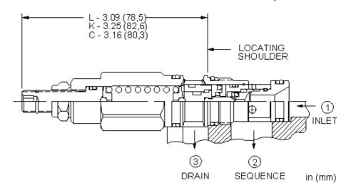
Direct-acting sequence valves will supply a secondary circuit with flow once the pressure at the inlet (port 1) has exceeded the valve setting. The pressure setting of a sequence valve controls the pressure at port 1 relative to the pressure at the drain (port 3).
