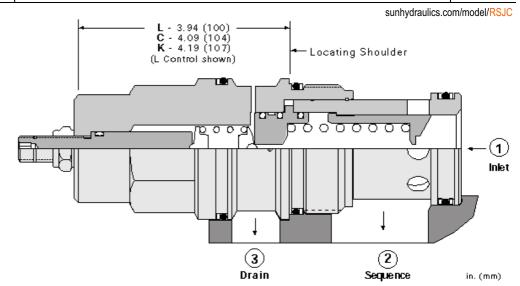
Pilot-operated, balanced piston sequence valves will supply a secondary circuit with flow once the pressure at the inlet (port 1) has exceeded the valve setting. The pressure setting of a sequence valve controls the pressure at port 1 relative to the pressure at the drain (port 3). These valves are insensitive to back pressure at port 2 (sequence), up to the valve setting. They may be used to regulate pressure in place of 2-port relief valves if there is pressure in the return line.
