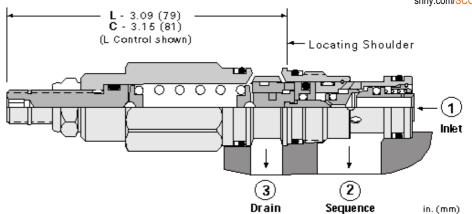
Direct-acting sequence valves with reverse-flow check will supply a secondary circuit with flow once the pressure at the inlet (port 1) has exceeded the valve setting. Additionally, these valves incorporate an integral check valve to provide reverse flow from port 2 (sequence) to port 1 (inlet). The pressure setting of a sequence valve controls the pressure at port 1 relative to the pressure at the drain (port 3).
