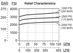
CAPACITY: 30 L/min. / CAVITY: T-163A
