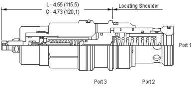
Pilot-operated, anti shock sequence cartridges limit maximum system pressure and also limit the rate of pressure rise. The valve opens and then ramps closed at a constant speed, independent of settings and flows. The adjust screw determines the maximum (relief) setting and the minimum (threshold) setting.
