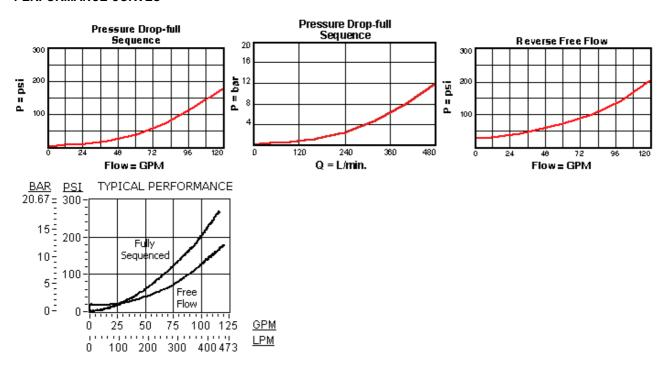
Anti-Shock, pilot-operated, balanced poppet sequence valve with drain to port 3
