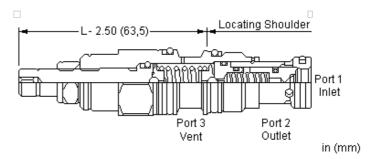
Pilot-operated, balanced poppet sequence valves will supply a secondary circuit with flow once the pressure at the inlet (port 1) has exceeded the valve setting. The pressure setting of a sequence valve controls the pressure at port 1 relative to the pressure at the drain (port 3). These valves are insensitive to back pressure at port 2 (sequence), up to the valve setting. They may be used to regulate pressure in place of 2-port relief valves if there is pressure in the return line.
