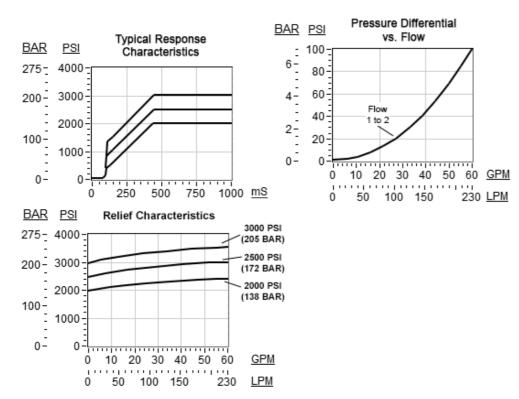
SERIES 4 / CAPACITY: 480 L/min. / CAVITY: T-19A
